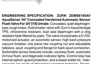
nal seals are made of chloramine resistant materials. Electrical box by others (see installation instructions for type and style). Note: Order power converter separate, one power converter operates up to eight valves.
